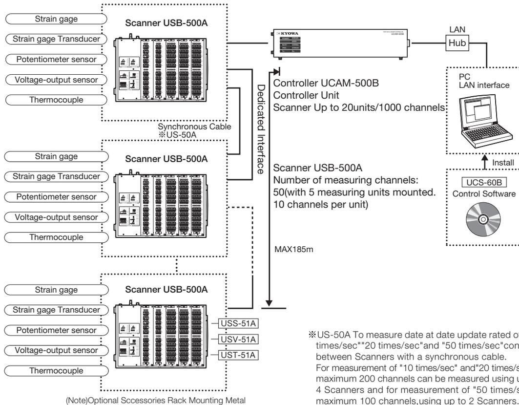
※US-50A To measure date at date update rated of "10 times/sec" "20 times/sec" and "50 times/sec" connect between Scanners with a synchronous cable. For measurement of "10 times/sec" and "20 times/sec", maximum 200 channels can be measured using up to 4 Scanners and for measurement of "50 times/sec" maximum 100 channels, using up to 2 Scanners.
