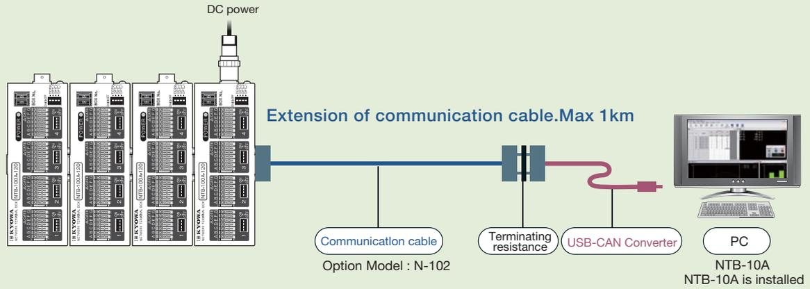
**Case B** 4 NTBs are distributed separately (\*Up to 8 units can be connected)
