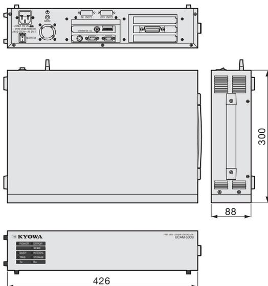
The UCAM-500B is a fast data logger system which can simultaneously sample variables at multiple points at a maximum rate of 50 times per second.
