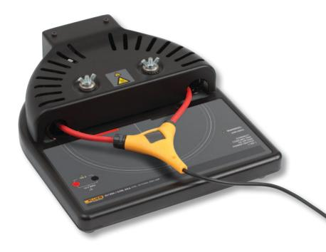
In each test case, the coil was loaded with a Fluke-381 Clamp or iFlex2500 Rogowski Coil.
