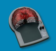
The **5500A/COIL 50-turn Current Coil** is a non-powered coil with a maximum compliance voltage rating of 3 volts RMS. At its rated current of 20 amps, it can calibrate clamp meters up to 1000 amps. It may run continuously to 11 amps, and must observe a 20% duty cycle from 11 amps to 20 amps.
