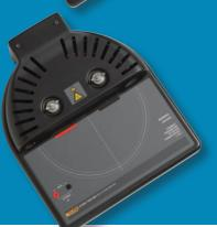
The **52120A/COIL6KA**, **COIL**, **50 TURN**, **6000 AMP** is a 12V-powered coil with a maximum compliance voltage rating of 4.5 volts RMS. Also convectively cooled, it may run continuously at 120 amps, allowing it to calibrate interruptible Rogowski coils, of lengths greater than 18 inches, at up to 6000 amps.
