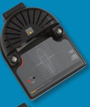
The **52120A/COIL3KA**, **COIL**, **25 TURN**, **3000 AMP** is a 12V-powered coil with a maximum compliance voltage rating of 4.5 volts RMS. With forced-convection cooling, it may run continuously at 120 amps, allowing it to calibrate clamp meters up to 3000 amps.
