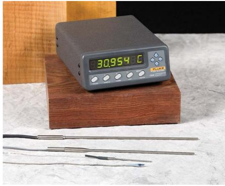
Hart's 1504 Tweener reads thermistors accurately to ±0.003 °C.
