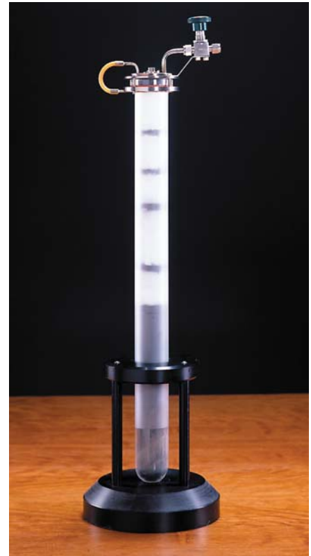
Open cells allow users to minimize the uncertainty from pressure corrections by regulating cell pressures themselves.
