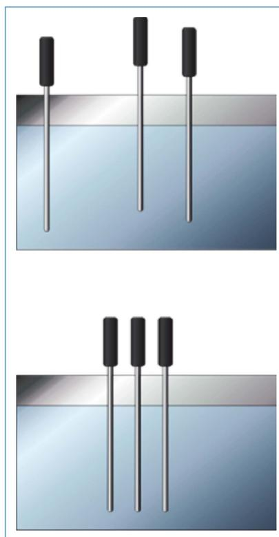
**Figure 2.** Though calibration baths are designed to provide excellent temperature uniformity, proper probe placement can further improve measurement uncertainty. Placing the probes in the bath at the same depth, close together and in the center of the bath will reduce the error caused by bath non-uniformity. Avoid letting the probes come in contact with the sides and bottom of the bath.
