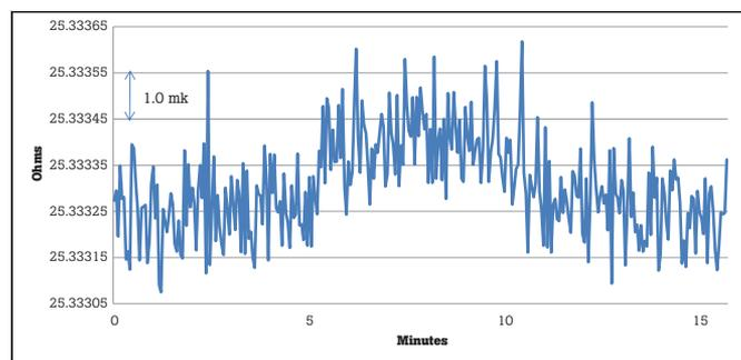
**Figure 1.** A new generation of Super-Thermometer with 10 times better noise characteristics than the previous generation clearly shows the effect of self-heating when excitation current is raised from 1 mA to 1.414 mA.
