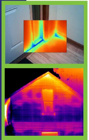
Inspecting to locate air leakage requires a 4 °F or higher temperature difference between inside and outside air, in order to get accurate readings. Air leakage can be into the building, as in the cold air shown leaking through the floor, or out of it, as in the warm air leaking out alongside the roof peak.
