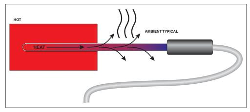
Figure 2, Stem conduction
