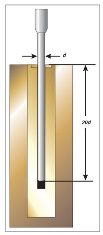
Figure 3. Recommended depth for probe immersion
