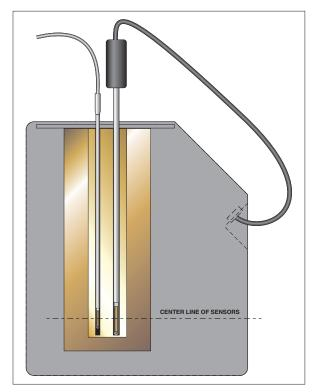
${\bf Figure~4.}$  Aligning the centers of the sensing element of the reference probe and the UUT
