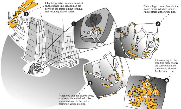
Figure 2. A worst-case scenario-potential arc blast sequence.
